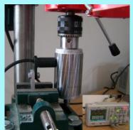
There is no output signal, when the rotor (see left picture) is measured with other sensors, except the optimized sensors: CYGTS101DC-S and CYGTS104X.
