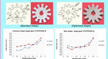
Testing with CYGTS104U-S, standard shape target gear (D=28, d=18, N=12,  $\theta$ =12°) and optimized shape target gear (D=28, d=18, N=12,  $\beta$ =5°)
